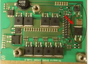
When you have a gysmi 190 product with this version of IMS Module (little diode), you **MUST** change the power block.
