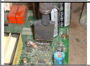
Put some tin on the connector, take off the power block after removing the screws and separate the diode bridge from the aluminium block
