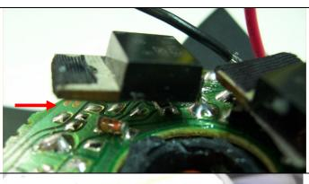
There is a risk of short circuit between the transistor metallic part and the components below.
