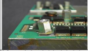
2. Consequently, the mechanical strains breaks the tracks where the bolts are soldered.
