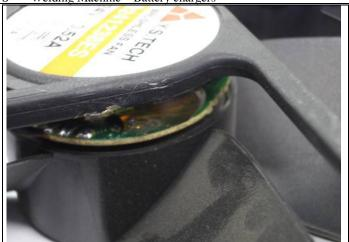
Insert some glue between the metallic part of the transistor and the fan PCB.
